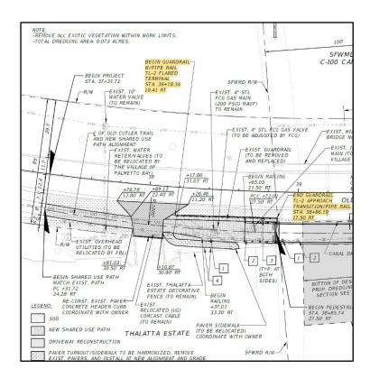
**Answer No.1:** The new shared use path will be located behind the new guardrail, which will require pipe rail to be installed.
