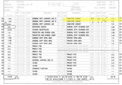
(1) EXISTING TO REMAIN (2) SAME BREAKER NEW LOAD. (3) NEW BREAKER NEW LOAD.
