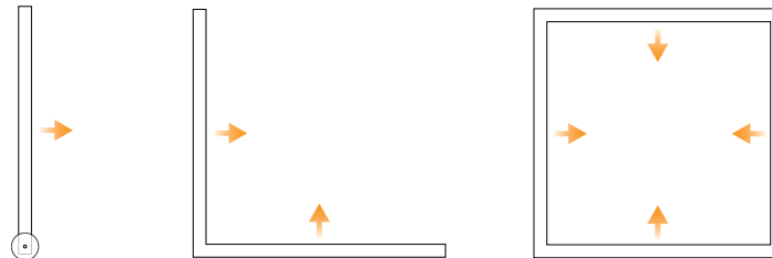
Straight Sections Light is thrown to right of the powerfeed (Can be reconfigured in field)
