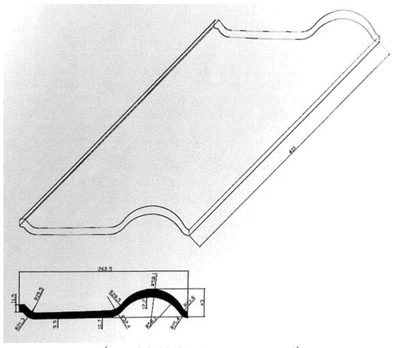
(DIMENSIONS SHOWN ARE IN MILLIMETERS)
