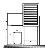
DIRECT MOUNT - STEEL STRUCTURE (36KSI) UNIT MUST BE ATTACHED TO ROOF STRUCTURE USING SIX GRADE 5 FASTENERS OF SIZE LISTED BELOW.
