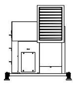
ISOLATION RAIL MOUNT UNIT MUST BE ATTACHED TO ISOLATION RAILS USING SIX GRADE 5 BOLTS LISTED BELOW. THE ISOLATORS WILL BE ANCHORED TO THE ROOF USING FASTENER SIZE LISTED IN TABLE.
