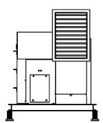
ISOLATION BASE MOUNT UNIT MUST BE ATTACHED TO ISOLATION RAILS USING SIX GRADE 5 BOLTS LISTED BELOW. THE ISOLATORS WILL BE ANCHORED TO THE ROOF USING FASTENER SIZE LISTED IN THE TABLE
