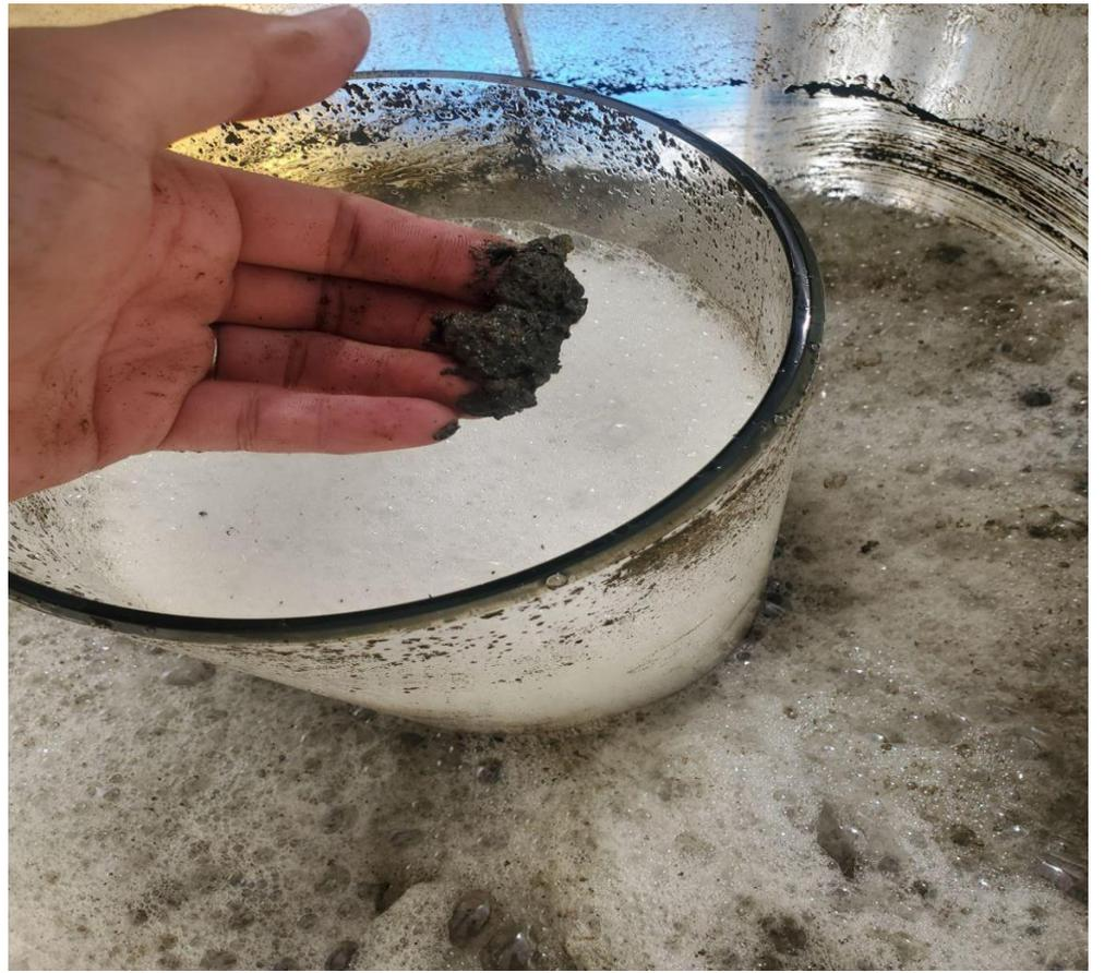
Skimmers separate significant pollution through millions of bubbles overflowing into the top hoppers and consolidating as concentrated sludge separated from cleaned oxygenated water which is returned to the environment.
