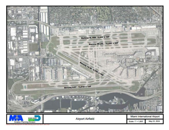
The four runways are flexible pavement facilities constructed with bituminous asphalt surfacing, over a compacted lime rock base sub-grade, and can be strengthened as necessary by additional overlays of bituminous asphalt to accommodate sustained operations by heavier aircraft in the future. All runways are grooved, permitting all-weather landing and optimal wet runway condition braking performance.
