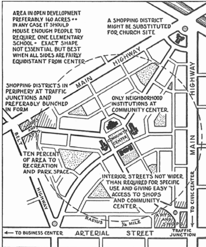
The Basic Components of Clarene Perrys Neighborhood Unit, from New York Regional Survey , Volume 7, 1929
