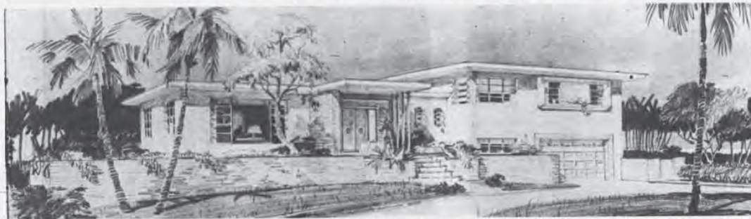
For this split-level house an artificial terrace was built up from fill, and blocked off with a low, decorative stone wall. This terrace supports the living area wing of the residence.
